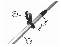
9. Slide middle main frame (Item 15) onto items 13 and 14 assembled in step 7 and lock together. Lubricate frame bars for best operation as shown in step 5.
