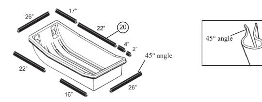
18. On the front of the fishhouse, start in the corners and work inward, snap the plastic trim seal on the canvas tent (Item 2) to the <u>lip</u> edge of the sled (Item 1). The tent (Item 2) will meet in the middle and should be free to open and close so it can be removed.
