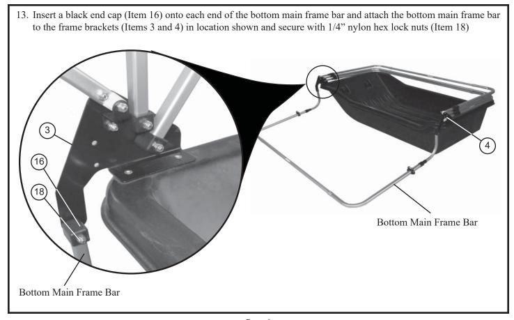
14. Set up main frame bars by grasping with both hands and pushing upward until button clicks into place. Start with bottom main frame bar and continue to the back main frame bar pushing lengthened bars into appropriate position.
